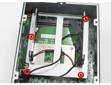
8. Then you can install the memory on the SO\_DIMM2 slot.
