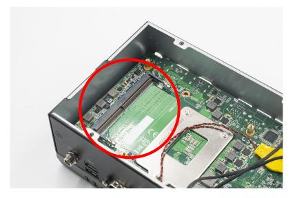
6. To install or replace the SO\_DIMM2, remove the 4 screw around the 2.5" slots first, and tilt up
