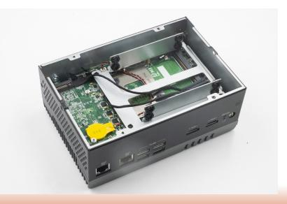
5. There are two M.2 slots and an InnoAGE HDR1 pinout on the board.
