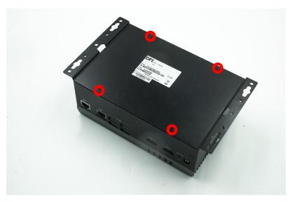
2. If you need to install or replace the CPU and 2nd memory, please also remove the three screws at each side of the box.
